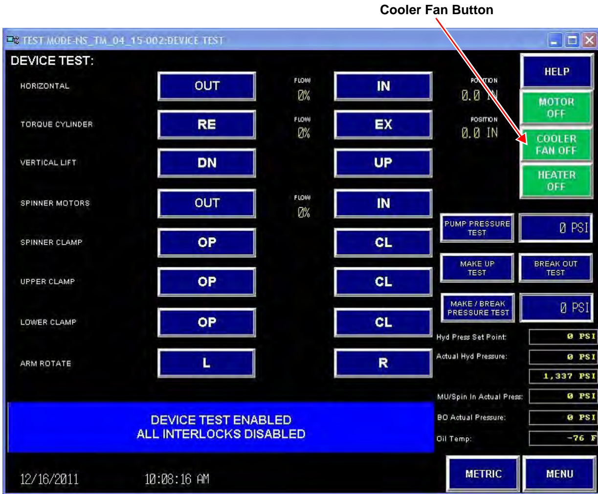
Figure 18: PLC test screen
