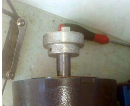
Figure 7: Coupling on the removed motor
