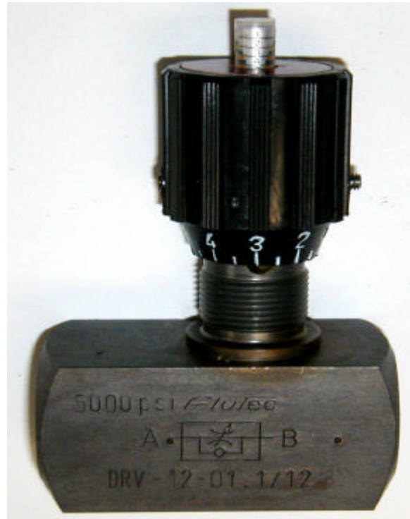
Flow control valve open Notice the flow indicator
