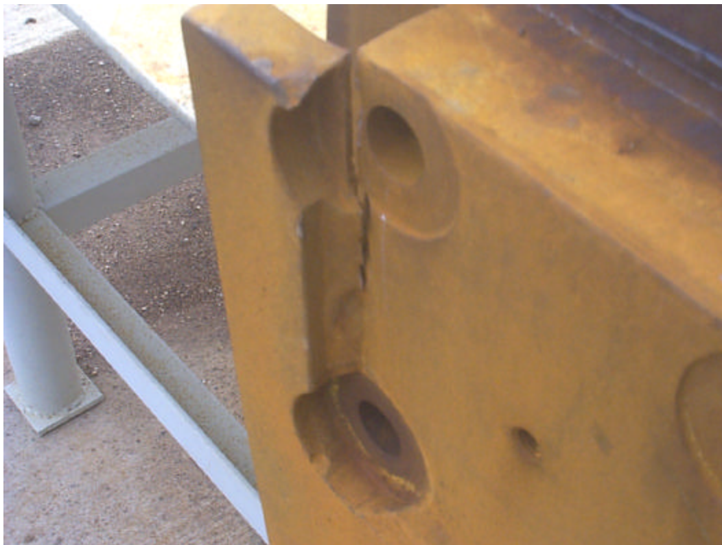
Figure 1: Typical Crack in a Slide
