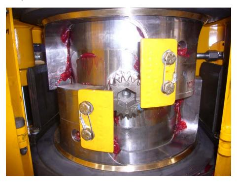
In addition to the safety wiring, the bolts must be loctited and torqued to 40 ft-lb. A kit part number AY15364 was created to include the necessary bolts, washers and safety wires as shown on the attached bill of material. This kit will be used for both the 3" and 4" actuators.
