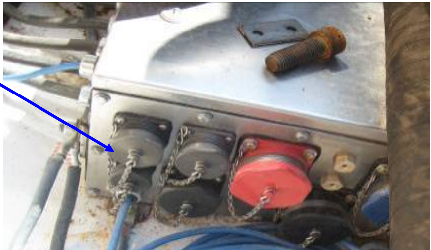
Lower Torque Guide J-Box assembled with the Plug Gland Plate Kit
