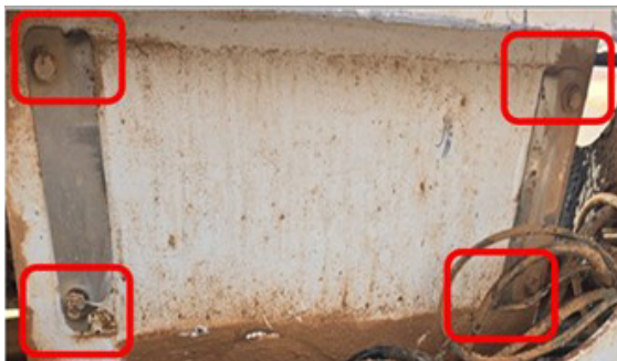
Figure 2: J-Box mounting welds failed and the J-box got crushed between the Carrier and Catwalk base
