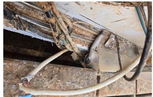
Figure 2: J-Box mounting welds failed and the J-box got crushed between the Carrier and Catwalk base
