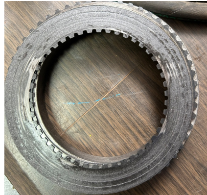
Figure 2: Worn friction disc
