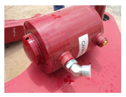
Replacement fittings from Canrig will include necessary orifice fitting. However, if orifice is missing, the technician can reuse the original orifice if it is not visibly damaged (orifice can be removed with hex wrench).
