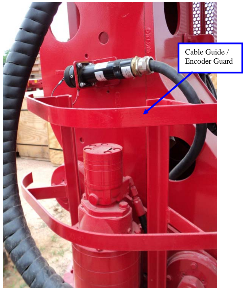
Figure 2: TM-80 Wrench with Cable Guide/Encoder Guard Installed
