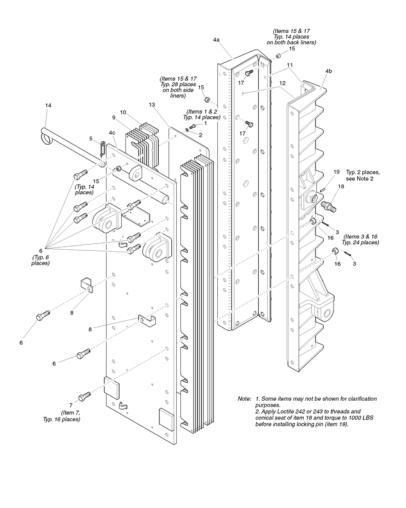
Revised version showing the slotted side plate mounting holes, notched side plates, 5-sided adjuster nuts, notched extend frame shim plates. Accumulator mount modifications are not shown but are to clear the new 5-sided adjuster nuts.
