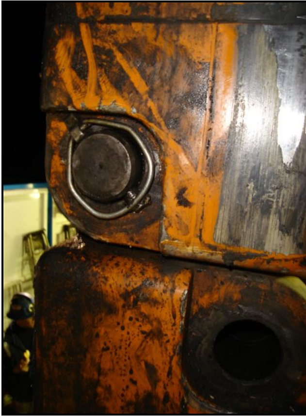
Figure 2: Intended use of the safety lynch pin (TESCO part number 13760)
