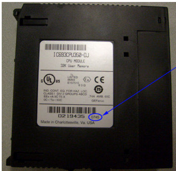
Figure 1 - Module's Date Code Location
