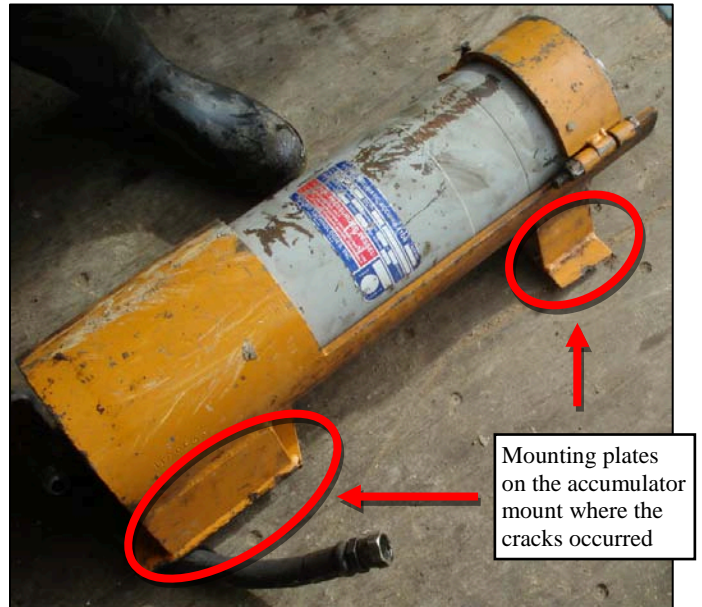
Figure 2: Counterbalance accumulator mount
