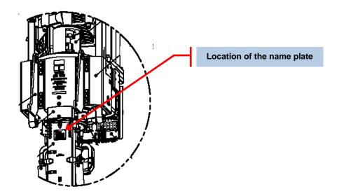
2. Confirm the gearbox housing serial number. It should be located as shown below.
