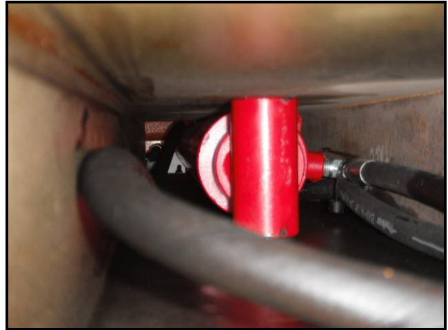
Figure 4: Lower rod retracted into the lift cylinder body
