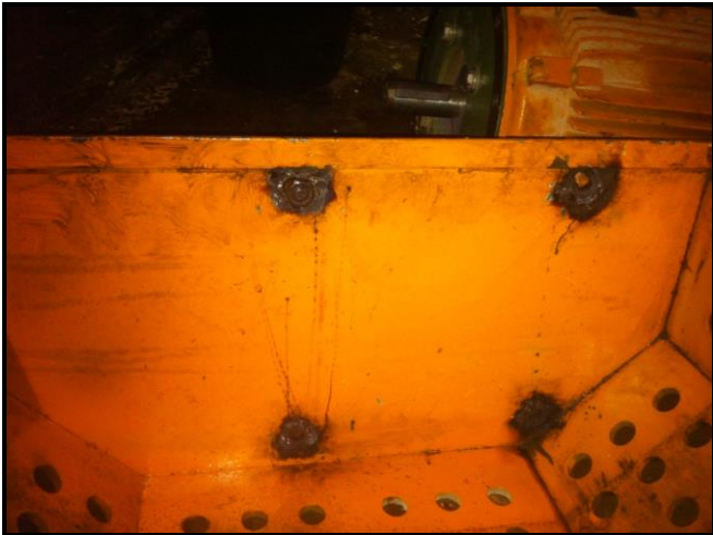
Figure 1: Welding of mounting nuts failed on ESI 500 Ton Top Drive
