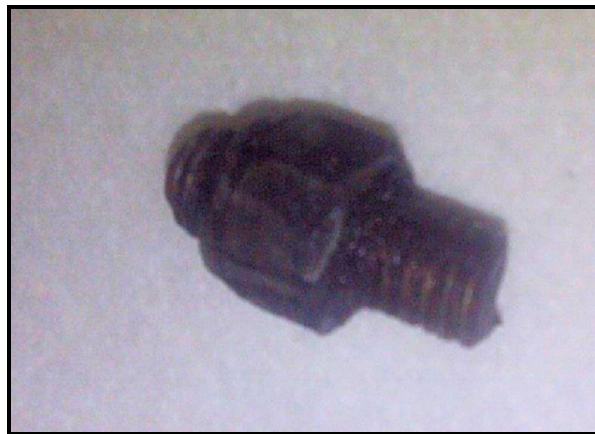
Figure 1: Recovered torque bushing extend arm pin
