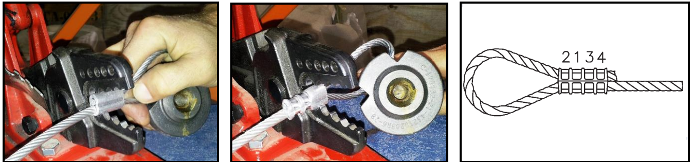
Figure 4: Using a bench tool to swage a compression sleeve
