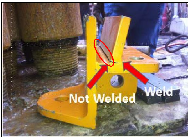
Figure 1: F-Clamp weld with one side of plate not fully welded
