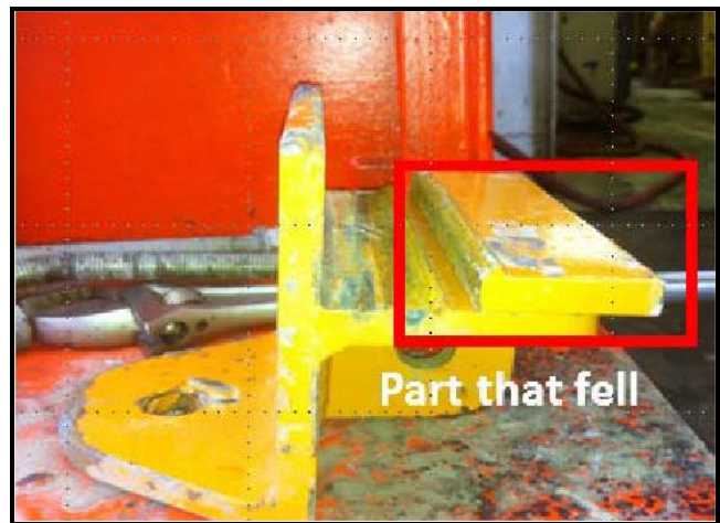
Figure 2: Plate from F-Clamp that fell onto the rig floor
