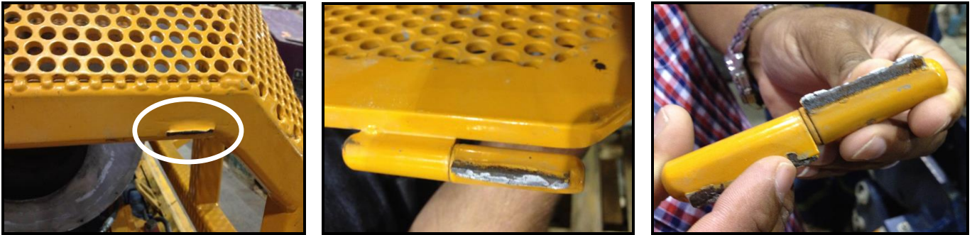
Figure 1: Hinge weld failure on the top door of the EMI guards
