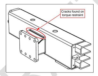
To prevent future occurrences of cracking on the torque restraint, TESCO developed a work instruction that describes the procedure to add reinforcing gussets to the torque restraint.
