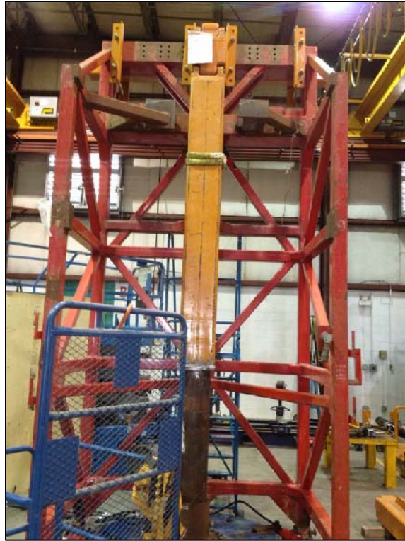
Figure 1: Torque arrest connection to the test frame
