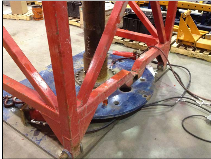
Figure 2: Coupled torque application cylinders of test frame
