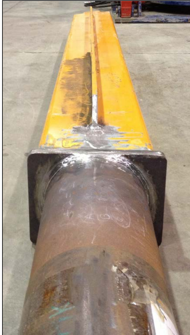
Figure 4: 9.6° permanent deformation in the torque track
