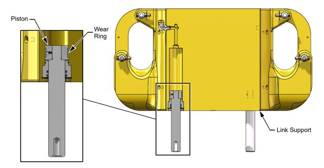
Figure 1: Upgraded piston cross section
